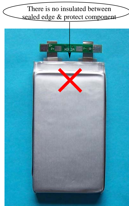
Fig.4. Schematic of wrong assembly
