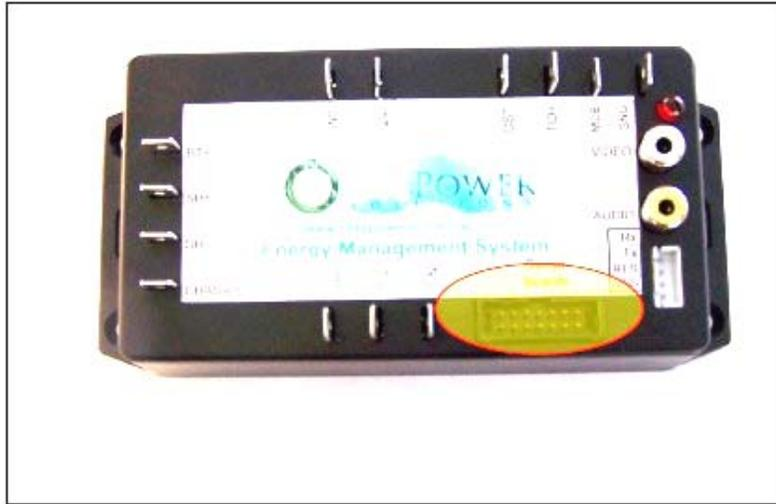
The sense board connector has a key to prevent it from being plugged in the wrong way.
