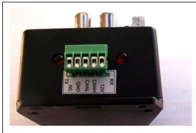
The green terminal block can be unplugged for easy wiring. Simply insert wires into the terminal block and tighten the screws.
