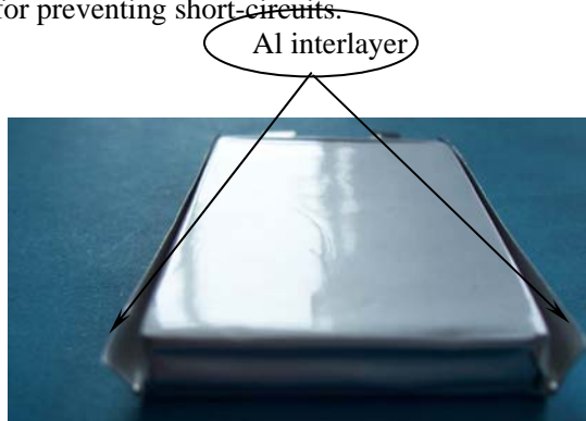
Fig.2. Single folding edge schematic of PL cells
