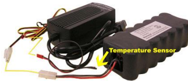
Temp sensor: attached to battery firmly
