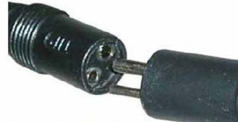
How to plug charger's [two pin universal male plug](#) to battery's [two pin universal female plug](#)
