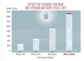
With the Cycle Satiator, you can program your primary profile to give an 80% charge, and have a secondary profile that does a 100% charge when you need full range. Then have the best of both worlds, a battery that lasts thousands of cycles but still goes the distance when you need it.
