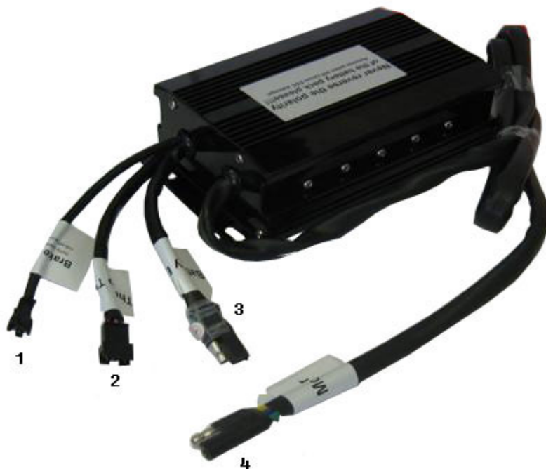
Pic2: 4 terminals from Controller unit .
