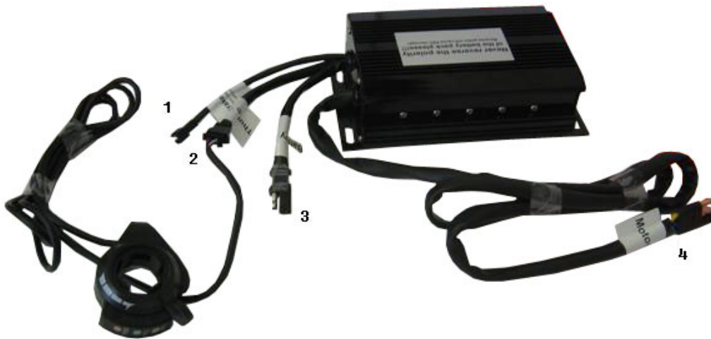
Pic3: How to connect the controller to thumb throttle unit
