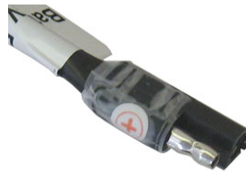
Pic 1: Positive Polarity label of Battery Terminal ( connector#3)
