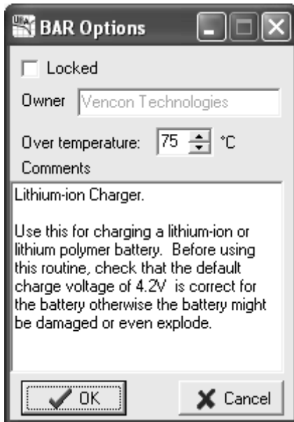
Figure 34: Maximum battery temperature in a BAR (mainly used for lithium cell charging).
