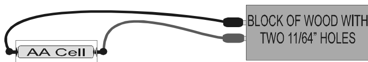
Figure 4: Using a block of wood to keep battery banana plugs from shorting.
