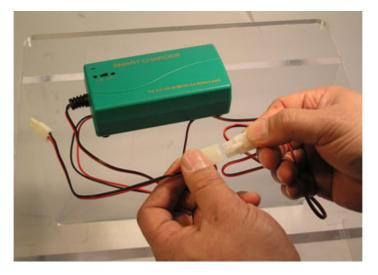
3. Connect standard mini female end of the connector adaptor to Charging Terminal of the pack (Standard mini male tamiya connector). Then connect the temperature sensor together.
