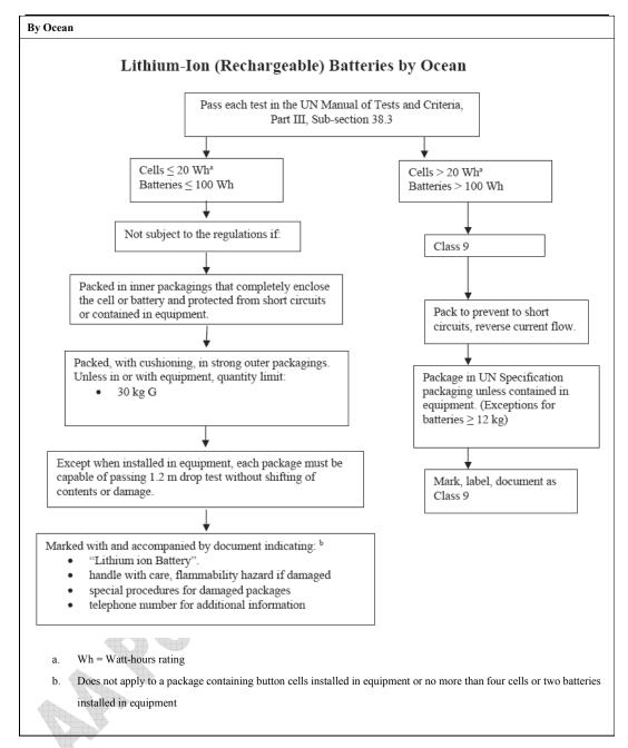
Separate Li-ion batteries when shipping to prevent short-circuiting. They should be packed in strong packaging for support during transport. In the case of transportation, confirm no leakage and no overspill from a container. Take in a cargo of them without falling, dropping and breakage. Prevent collapse of cargo piles and wet by rain. The container must be handled carefully. Do not give shocks that result in a mark of hitting on a cell. Please refer to Section 7-HANDLING AND STORAGE also.
