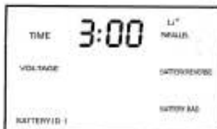
Fig 2H Battery Bad
