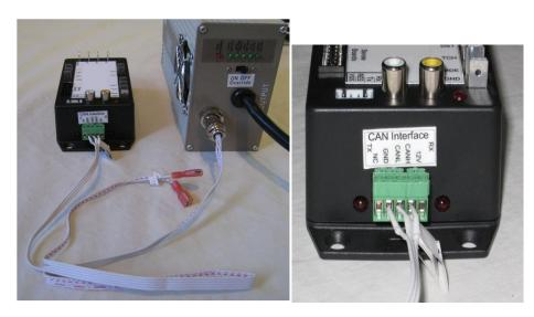
If both the CAN communication and the digital inputs are connected CAN communications will take priority over the digital input for charge control. CAN communications requires the optional CAN board be installed on the BMS CPU.
