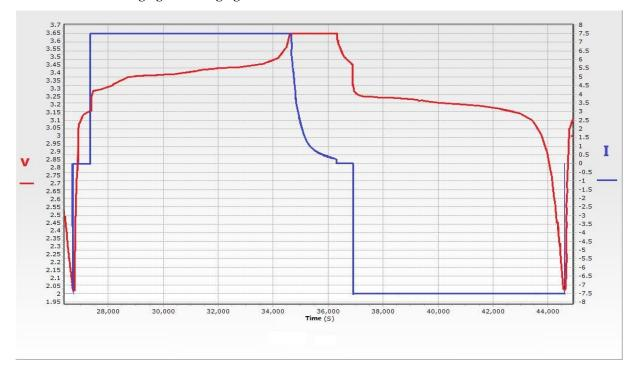
40152S discharging and charging curvs at discharging rate of 1C:
