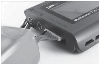
Battery Connection Diagram
