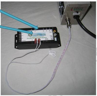
5.3 For a CAN communication connection connect the CANH, CANL and CAN GND to the matching connection on the CAN connection on the EMS CPU. The white connector may be cut off of the cable; however, note which wires are which before doing so.
