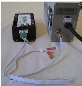
5.4 If both the CAN communication and the digital inputs are connected CAN communications will take priority over the digital input for charge control. CAN communications requires the optional CAN board be installed on the EMS CPU.
