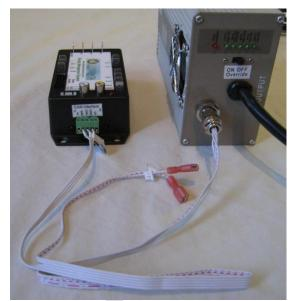
5.4 If both the CAN communication and the digital inputs are connected CAN communications will take priority over the digital input for charge control. CAN communications requires the optional CAN board be installed on the EMS CPU.
