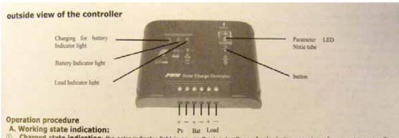
Charged state Indication: the solar indicator light is on, as the input voltage of solar battery panel reaches a certain point. The indicator light flashes slowly, as the storage battery is charging. The indicator light will flash quickly, as the system is over voltage.
