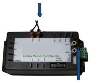
Connect the video output to a screen. The above will be displayed. "E.M.S. – 0"will be displayed. This is the number of sense boards the CPU has detected.
