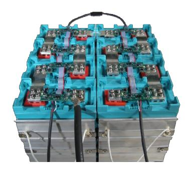
The above is an example of a completed EMS-8 setup. Up to 156 boards can be added to the string
