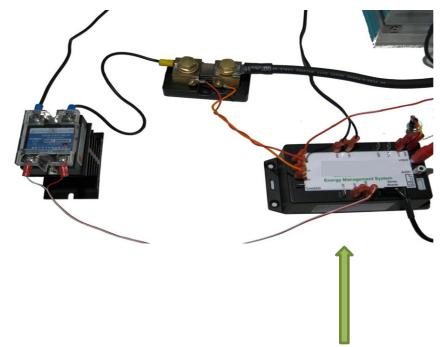
In this example a solid state relay controls the chargers output to the battery pack. The relay is controlled by the OV output which turns on the relay during normal conditions and turns it off during a high voltage cell situation to prevent over charging.
