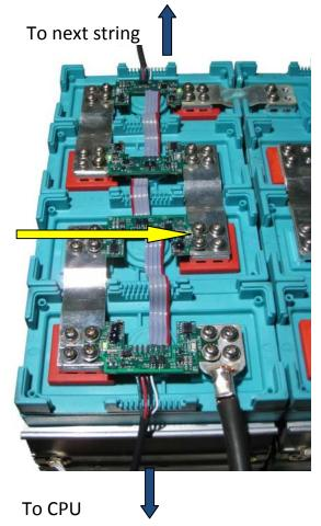
Connect the battery pack in series and install any other electrical hardware before installing the sense boards.
