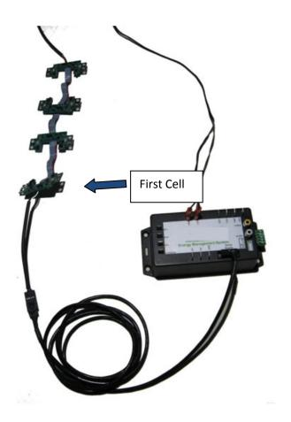
The sense boards are connected in four cell strings. Plug the first string in to the main wiring harness and connect the harness to the CPU. The first board connected to the CPU will be cell #1. The sense boards can be wired from either the negative most battery to the positive most battery, or the positive most battery to the negative most battery. The string must follow the series connection of the batteries.
