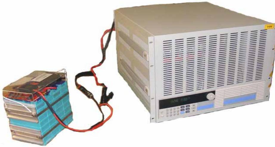
**How to connect with excluded standard Anderson plug & excluded DC Programmable Electronic load: 0-240A / 0-150V / 3600W --- M9717**
