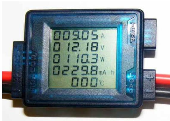
**Voltage (V) , Current (A), Power (W), Electronic Charge (mAh) parameter demonstrated while being charged by Smart Charger (10 A, Watt-Meter Built In, Large Alligator Clip plug) for 12.8V LiFePO4 Battery Pack Worldwide use**
