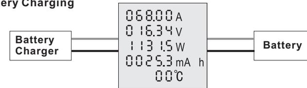
With a battery charger on the SOURCE side and battery pack on the LOAD side, the meter shows the charging current into the battery, the voltage and charging power at the battery and accumulate the charge (mAh) into the battery.
