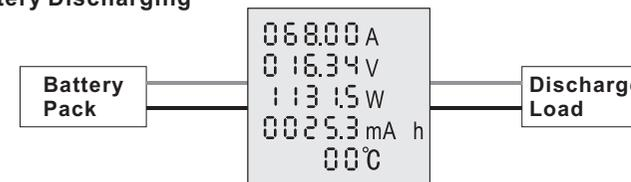
When the battery is discharged, the meter indicates the total charge (Ah) the battery delivered to the load as well as current, voltage and discharging power..
