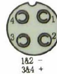
Pin assignment for 14.8V 6.0A Li-Ion smart charger charging terminal
