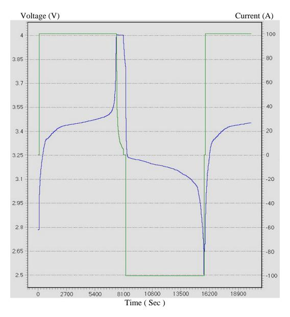
Charge/Discharge curve by CC/CV mode
