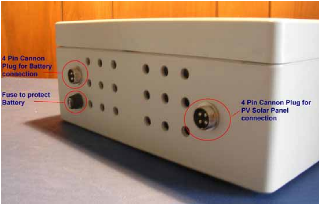
Back View: 20.0A fuse installed for protect battery, Solar Panel and Battery socket
