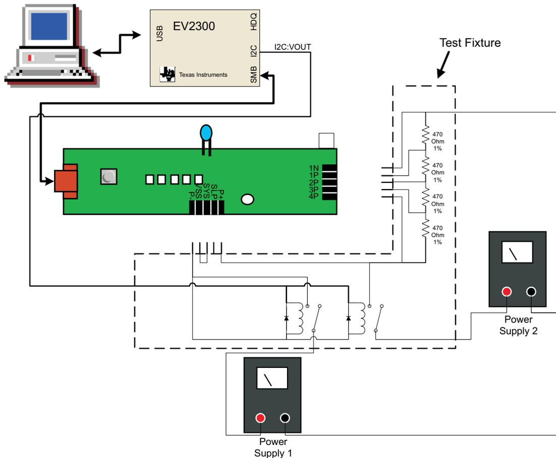
bqTester single site software from Texas Instruments (TI) is designed to calibrate and program electronic smart battery modules based on the bq20z70, bq20z80, bq20z90, and future advanced battery gas gauges. The bqTester works with the TI EV2300 USB-based PC interface board for battery fuel gauge evaluation. The bqTester is open-source software and can be modified to suit the user's requirements.
