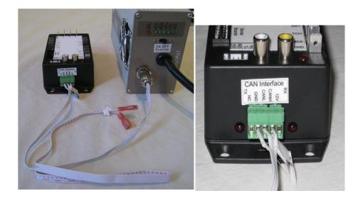
If both the CAN communication and the digital inputs are connected CAN communications will take priority over the digital input for charge control. CAN communications requires the optional CAN board be installed on the BMS CPU.
