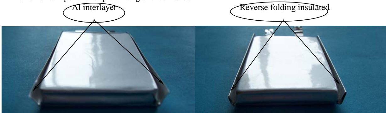
Fig.2. Single folding edge schematic of PL cells
