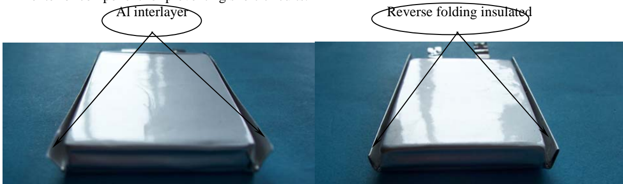
Fig.2. Single folding edge schematic of PL cells
