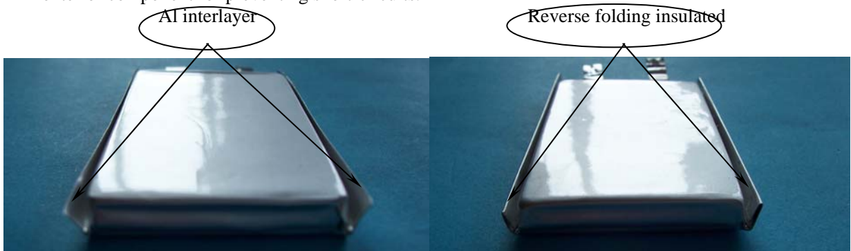
Fig.2. Single folding edge schematic of PL cells
