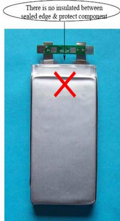
Fig.4. Schematic of wrong assembly
