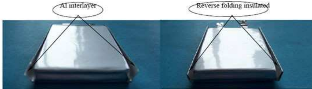
Fig.2. Single folding edge schematic of PL cells
