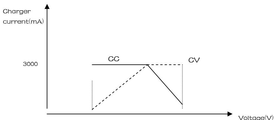
2.1.1 Its output voltage is 29.4V+/-1.0% at standby.
