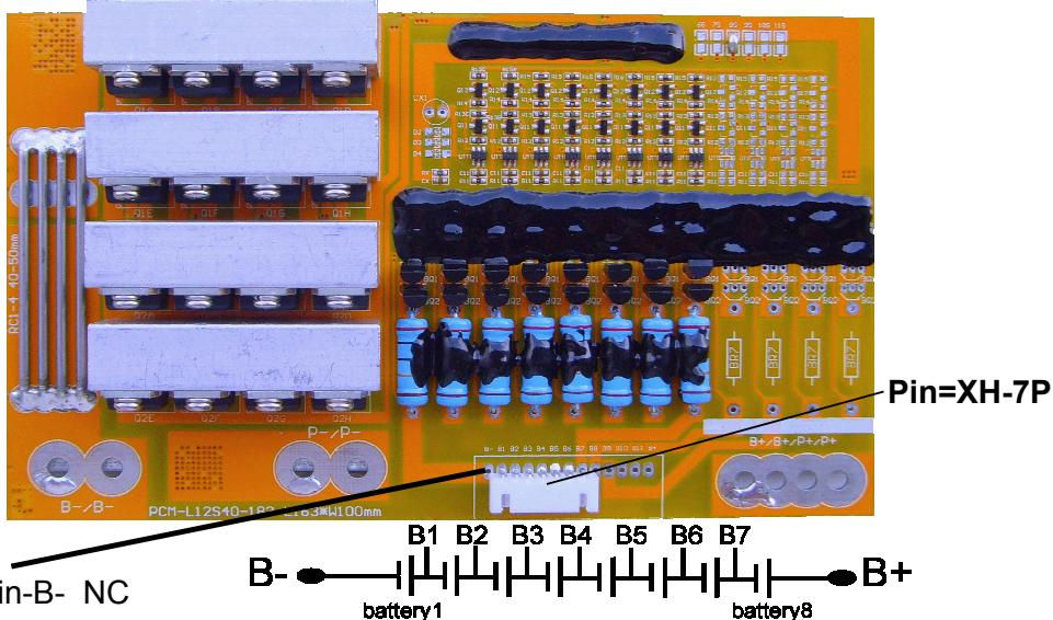
Important: Must connect from B-/B1 to B7/B+ in sequence, should not connect in random sequence. Otherwise , you will damage the circuit board.
