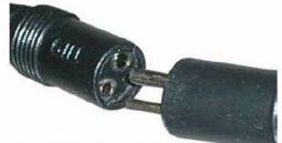
How to plug charger's two pin universal male plug to battery's two pin universal female plug
