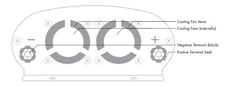
High Speed Fan – Keeps the inverter circuitry cool. The fan operates when the inverter is powered on. To avoid unnecessarily draining of the battery, turn off the inverter when it is not in use.
