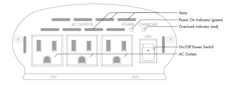
$\mathsf{ON}/\mathsf{OFF}$  Switch – Controls operation of the inverter. The below indicators operate when the switch is  $\mathsf{ON}.$
