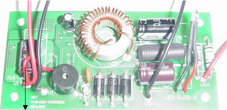
Connect SW1-1 to SW1-2, output voltage is 12.0V
