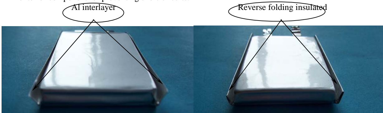
Fig.2. Single folding edge schematic of PL cells
